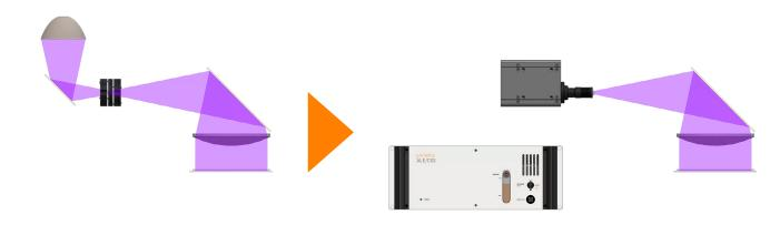
Our High-Power UV-LED Exposure System ALE/1C follows a distributed design approach with a Control Subsystem (CSS) separated from a small footprint Exposure Subsystem (ESS) to be directly integrated into collimated exposure equipment, i.a., Mask Aligners.
