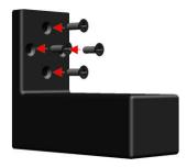
3.5 Place the screws into the according threads in the back of the MONARCH camera and screw in tightly.
