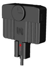
6.3 Place the Tripod Add On top of the Cable Add On so the slots are aligned.
