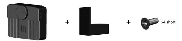
3.4 Insert the 4 short screws into the designated slots in the back of the Tripod Add On
