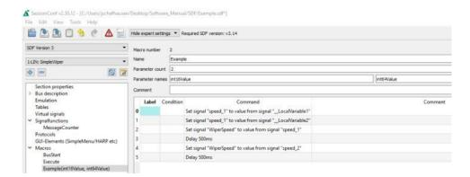
A macro can receive up to 10 parameters when called. In the macro definition, you can give these parameters names, which are then displayed on the left in the menu tree in brackets after the macro name. The parameters end up in the signals \_LocalVariable1...10 of the called. If no parameters or less than 10 parameters are are passed, the remaining LocalVariableX signals receive the value 0.
