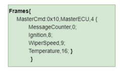
The frame is structured as shown in the following graphic. The frame defined in the LDF is recognised with the identifier with ID = 0x10 and the signals can be mapped from the 4 databytes.
