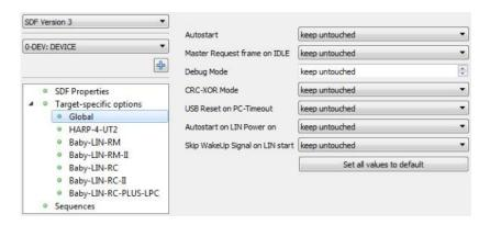
The target-specific options can be set using the SimpleMenu. Right click on the connected device and click on "Target configuration". In the following dialog you can change the values in the device. For comparison reasons the preset values of the SDF are shown.
