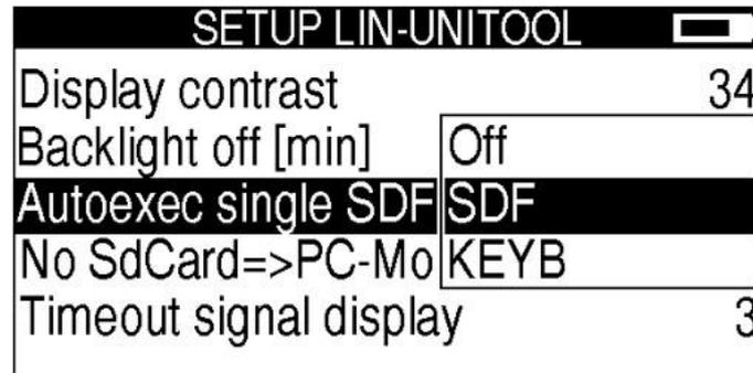
Press "ESC" to exit the menu and press "MEM" to save the changes. If you now switch the HARP-5 off and then on again the autostart macro should be executed and the SDF or Keyboard menu will be shown.
