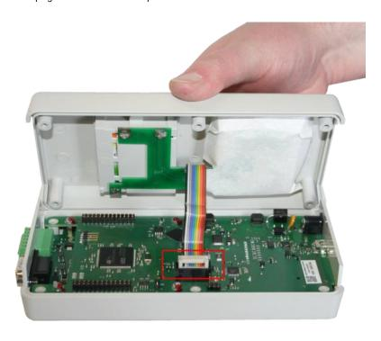
Grab the circuit board on its sides and carefully pull it straight up until it is detached from the case.
