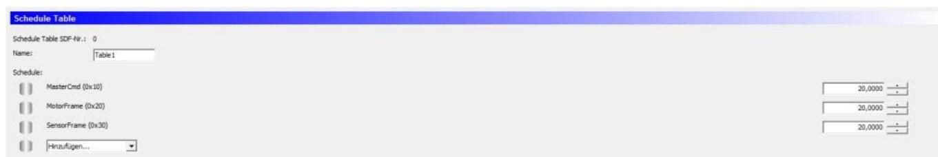
A Schedule Table is always selected as active and is executed by the master. The master places the corresponding frame headers on the bus and the publisher assigned to this frame places the corresponding data section + checksum on the bus.
