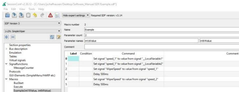
A macro can receive up to 10 parameters when called. In the macro definition, you can give these parameters names, which are then displayed on the left in the menu tree in brackets after the macro name. The parameters end up in the signals `_LocalVariable1...10` of the called. If no parameters or less than 10 parameters are passed, the remaining `_LocalVariableX` signals receive the value 0.
