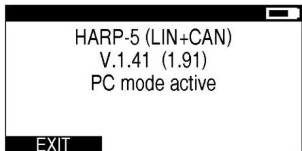
If the PC mode is currently enabled, simply press the "F1" key to exit the PC mode again.
