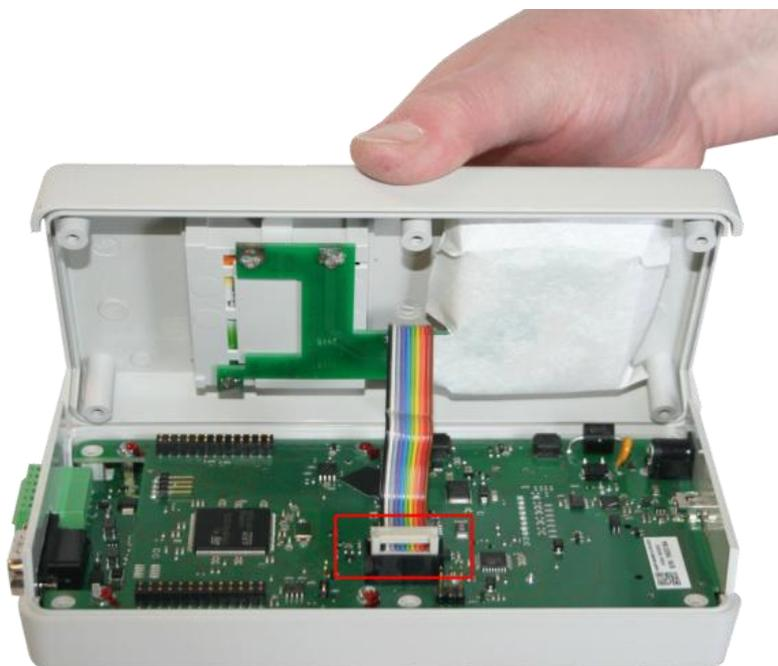
Grab the circuit board on its sides and carefully pull it straight up until it is detached from the case.
