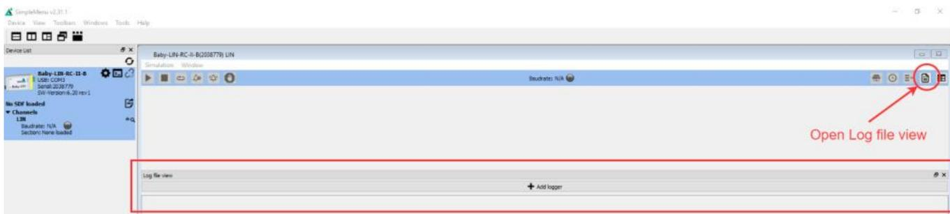
After opening the Log file View, you can now add a logger. Adding the logger opens the Logging Configuration. Existing LOG configurations can be loaded or new ones can be created.
