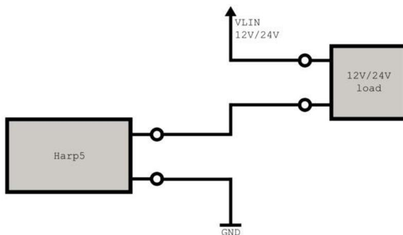
If a load is connected, please make sure the maximum current through the output of the HARP-5 is lower than 200 mA.
