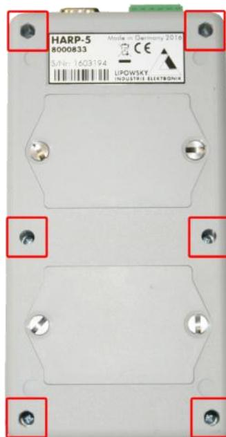
Open the case carefully until you can unplug the ribbon cable. Then place the back side of the case somewhere safe.
