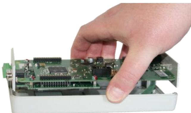
Lay down the circuit board and hold up the front side of the case.
