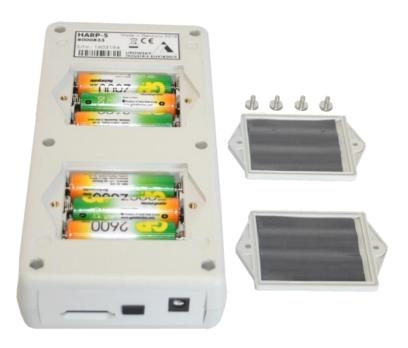
Now you can remove the old batteries and insert six new rechargeable batteries (Check the type above).
