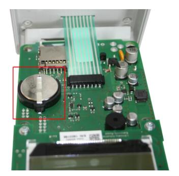
Now you should be able to see the button cell within the battery holder under the display on the right side.
