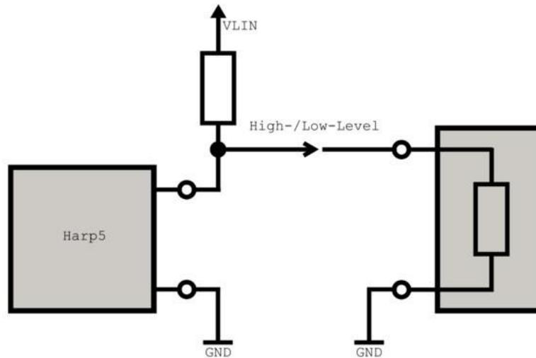
The calculation of the pull-up resistor value must meet two criteria:
