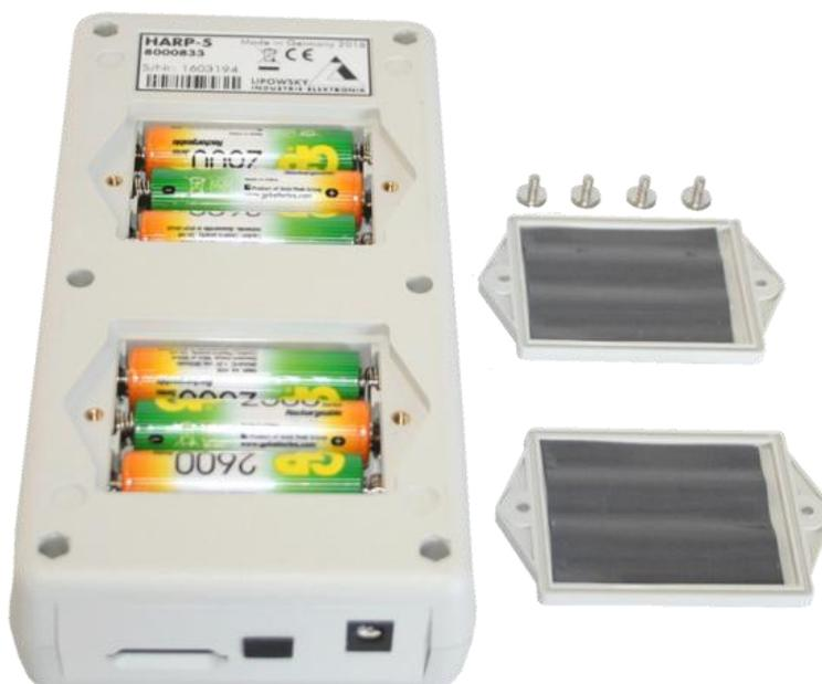
Now you can remove the old batteries and insert six new rechargeable batteries (Check the type above).
